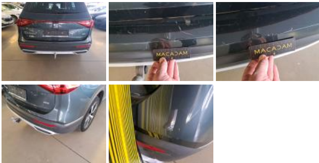
Bumper trim R, Dent(s) and scratch(es), Smart repair
