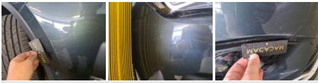
Bumper spoiler F, Scratch(es), Replace
