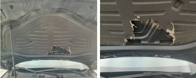
Front Bonnet / Insulation / Replace-tear
