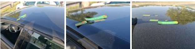
Roof, Dent(s), Repair and paint (complete)
