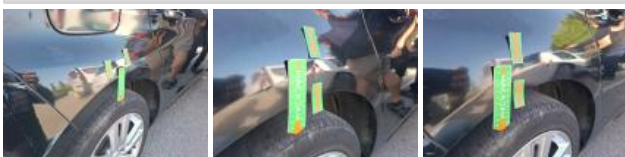
Wing RR, Dent(s), Repair and paint (complete)
