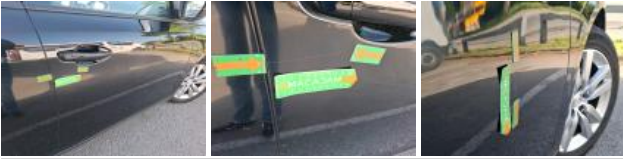
Roof pillar R, Dent(s), Repair and paint (complete)
