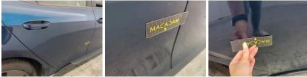
Outer door handle RR, Scratch(es), Repair and paint (complete)
