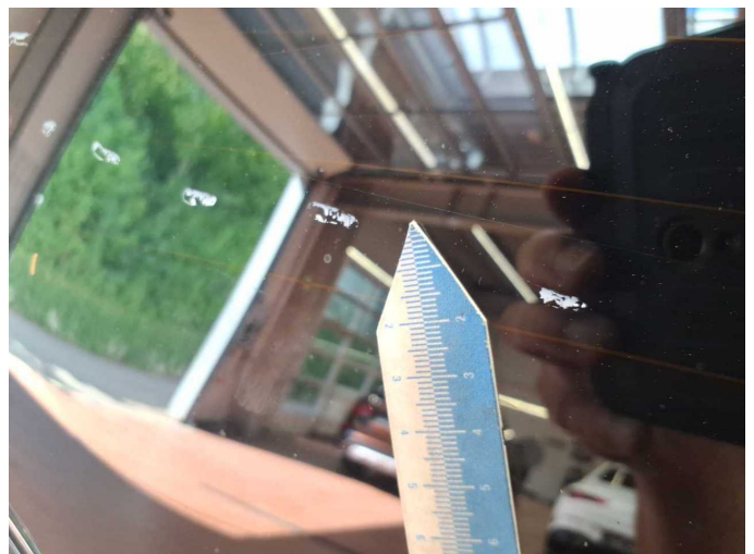
Damage 6: Vehicle glazing: Rear window black glass (Optischer Mangel) - Scratch(es) - Loss in value
