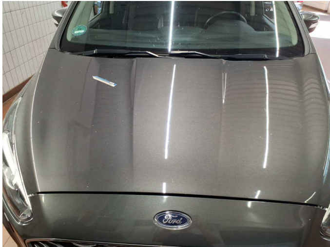
Damage 8: Bonnet: Bonnet - Dent / paintcoat damage - Paint
