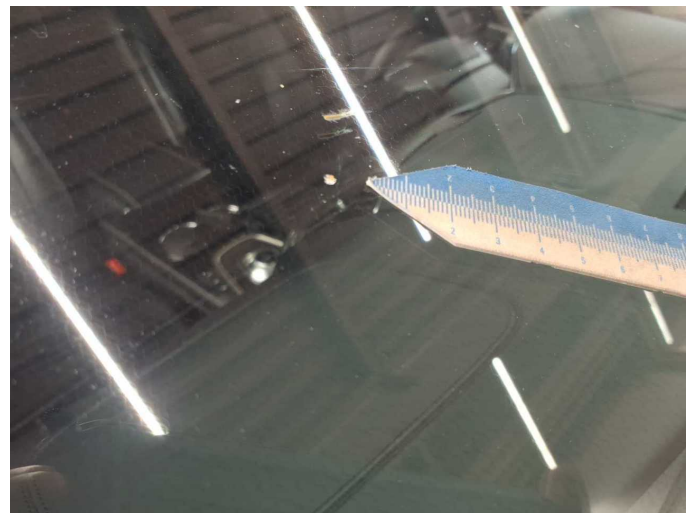
Wear and tear 1: Vehicle glazing: Windscreen (Abplutzer) - Stone chips - No deduction
