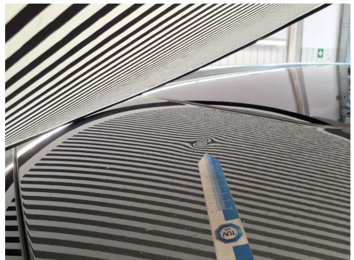
Damage 7: Roof: Roof - dent(s) - Paint
