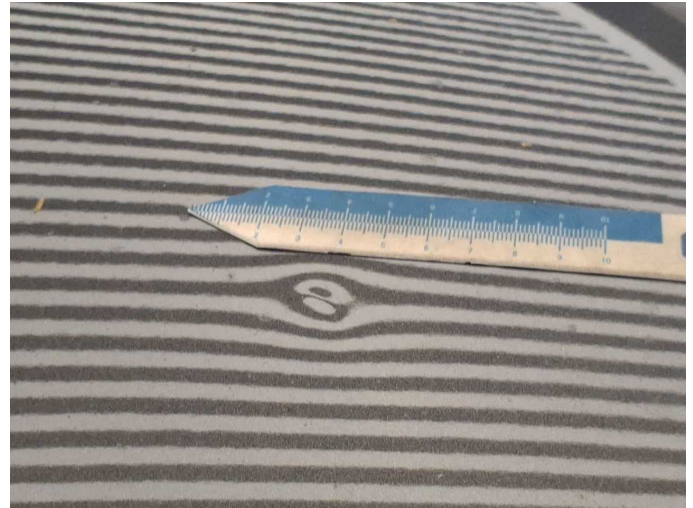
Damage 8: Bonnet: Bonnet - Dent / paintcoat damage - Paint
