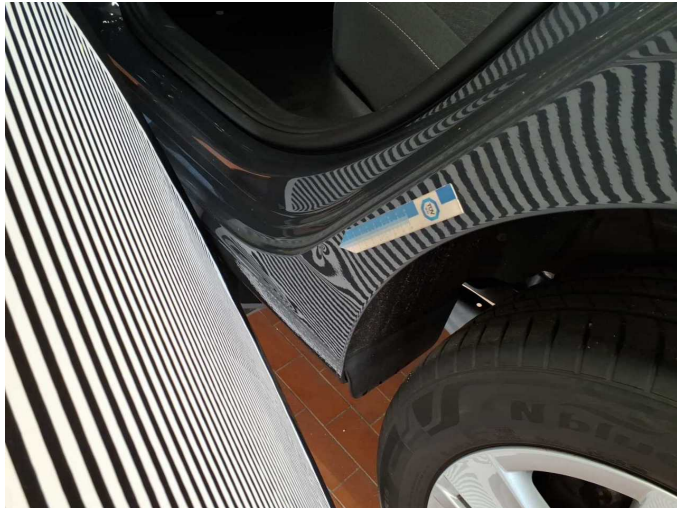
Damage 6: Side panel - rear left side: Elbow - Dent / paintcoat damage - Paint
