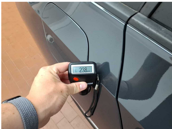
Repainting 1: Side panel - rear right side
