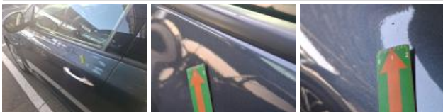
Door RL, Bad repair, Paint
