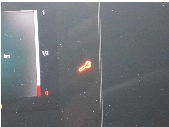
Damage 2: Misc.: Inspection / maintenance - Due - Perform diagnosis
