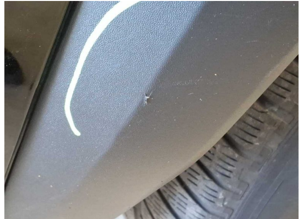
Damage #3: Side panel - rear right side: Wheel well extension - Scratched - Loss in value
