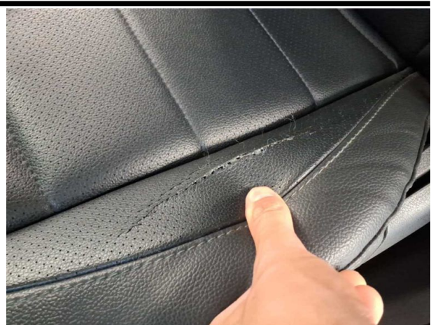
Damage #5: Seat - front: Seat cover - left side - Damaged - Replace
