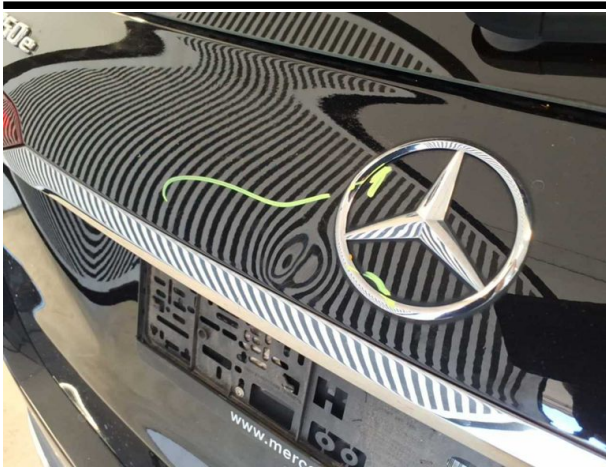
Damage #8: Boot lid / rear door: Boot lid - Dent / paintcoat damage - Repair and paint
