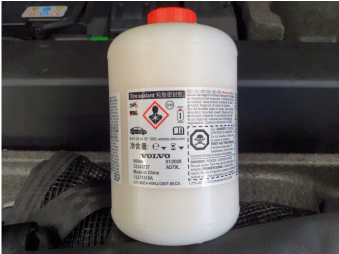
Damage 1: Equipment: Tirefit filler - Expired - Replace
