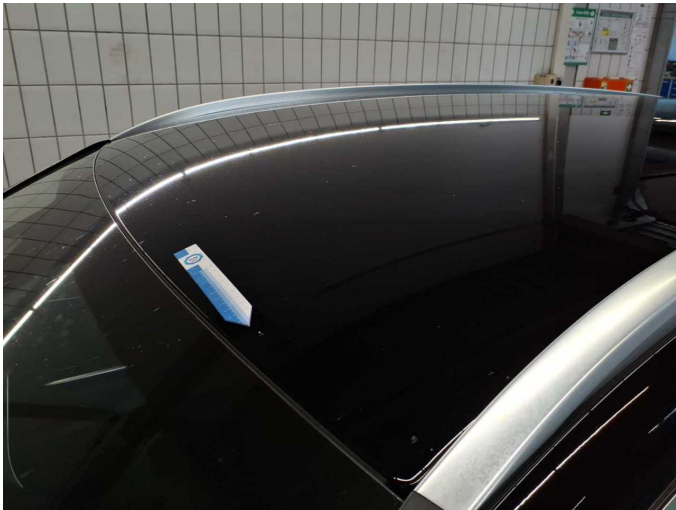
Wear and tear 7: Roof: Roof - Stone chips - No deduction
