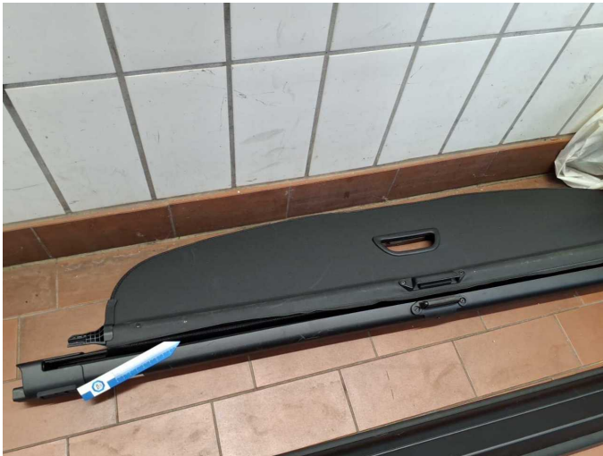
Damage 6: Interior: Boot cover / roller cover - Broken / torn - Replace
