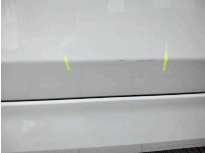
Damage 3: Door - rear right side: Door - Damage caused by marten / rodent - Smart repair
