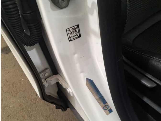
Damage 3: Sill - right side: Sill - Dent / paintcoat damage - Paint
