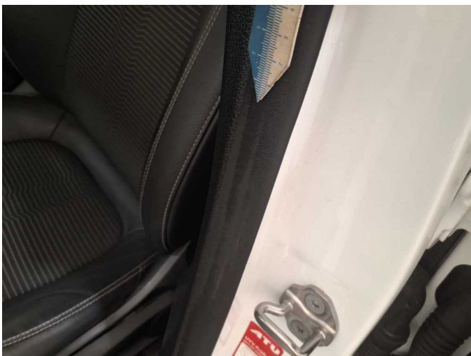
Damage 2: Door - front left side: Door seal - Damaged - Replace
