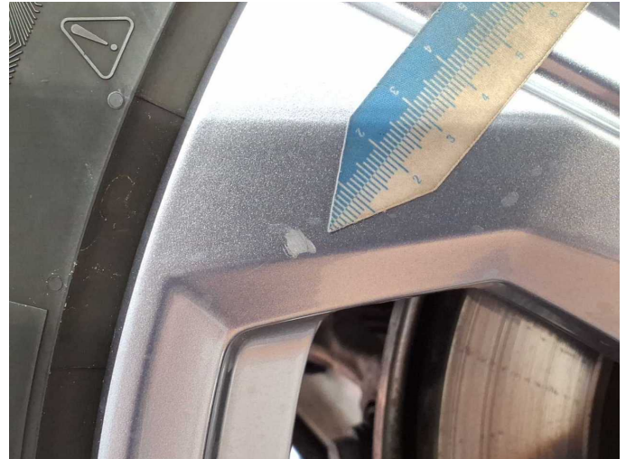
Damage 1: Wheel / tyres: Alloy rim - rear right side - Scratch(es) - Loss in value
