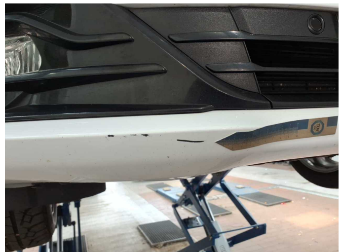
Damage 8: Front bumper: Front bumper - Scratch(es) - Paint
