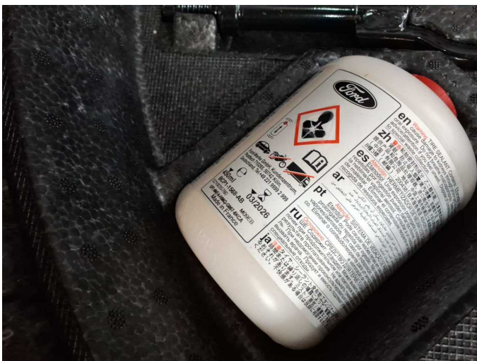
Damage 2: Equipment: Tirefit filler - Expired - Replace
