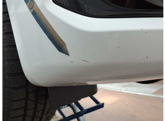
Damage 8: Front bumper: Front bumper - Scratch(es) - Paint
