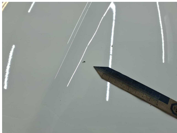
Damage 9: Bonnet: Bonnet - Stone chips - Paint
