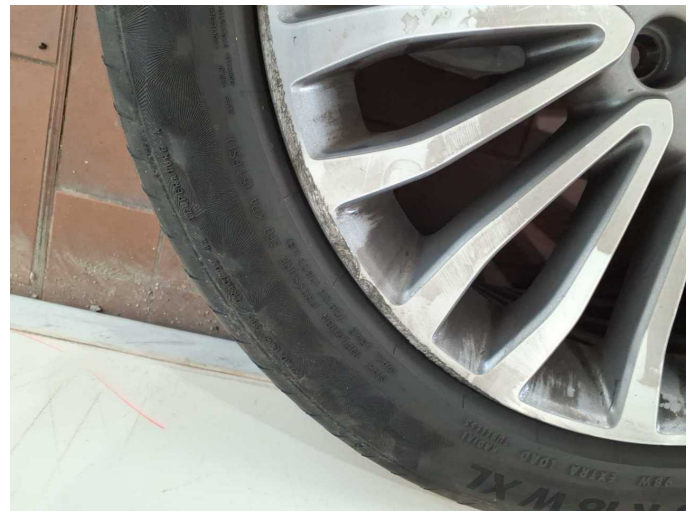
Damage 7: 2nd wheel set: 2 alloy rims - Scratched - Replace
