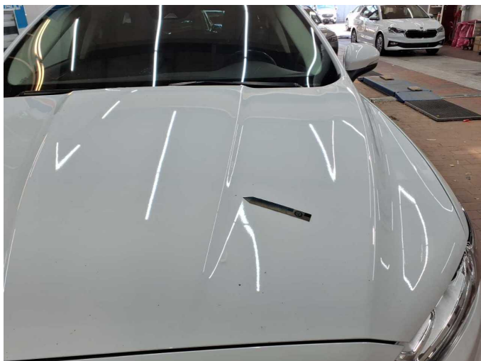
Damage 9: Bonnet: Bonnet - Stone chips - Paint
