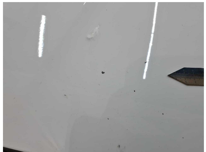
Damage 9: Bonnet: Bonnet - Stone chips - Paint
