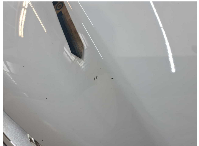
Damage 9: Bonnet: Bonnet - Stone chips - Paint
