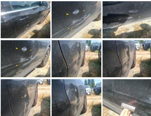
Door RR, Dent(s), Repair and paint (complete)
