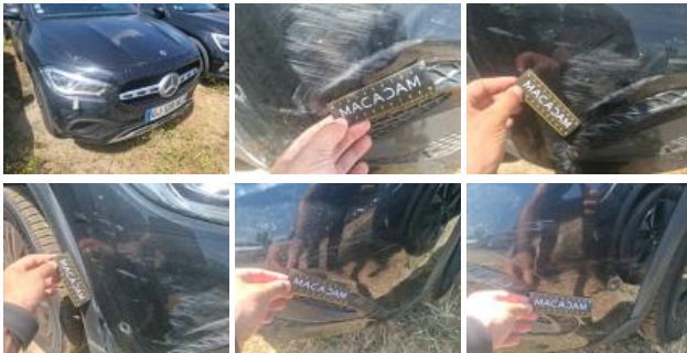
Door FR, Dent(s), Repair and paint (complete)
