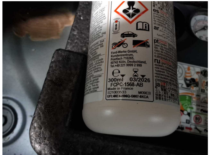
Damage 1: Equipment: Tirefit filler - Expired - Replace
