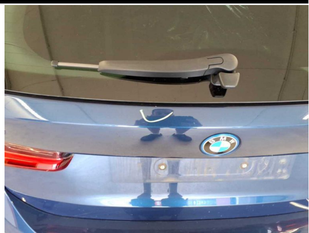
Damage #6: Boot lid / rear door: Boot lid - Scratched - Smart repair
