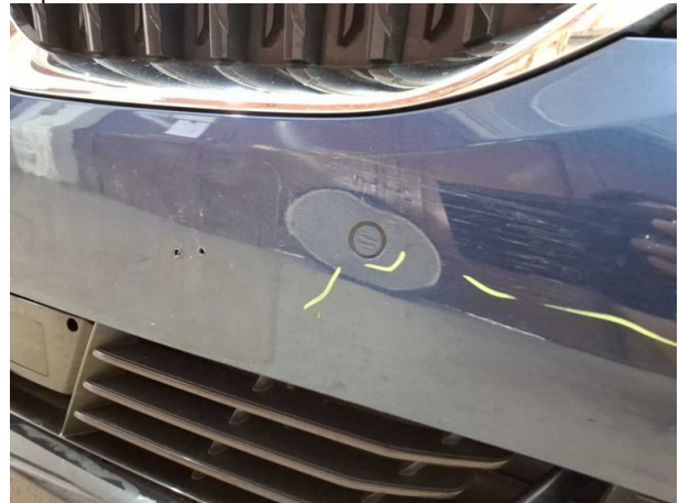
Damage #11: Front bumper: Front bumper - Damaged - Replace
