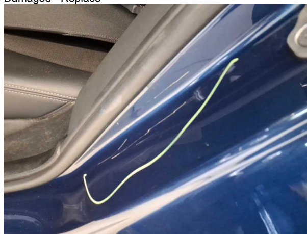
Damage #3: Side panel - rear left side: Sill - Scratched - Smart repair
