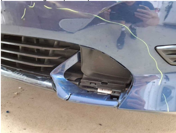
Damage #11: Front bumper: Front bumper - Damaged - Replace
