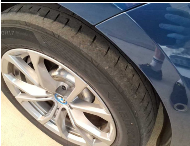
Damage #5: Measurement: Undercarriage - Malposition - Set / adjust
