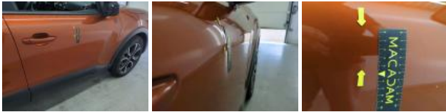
Mirror side repeater R, Broken, Replace
