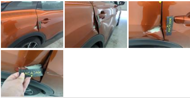
Wheel arch cover RR, Scratch(es), Replace
