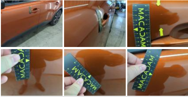
Door RL, Scratch(es), Repair and paint (complete)
