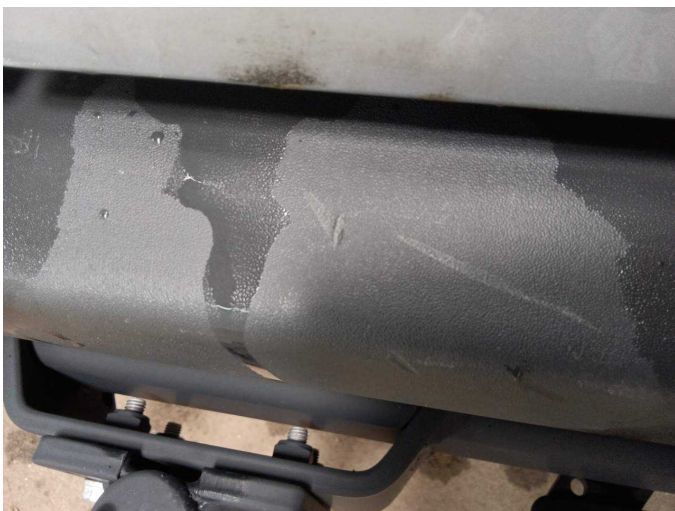
Damage 3: Rear bumper: Rear bumper - Scratched - Replace
