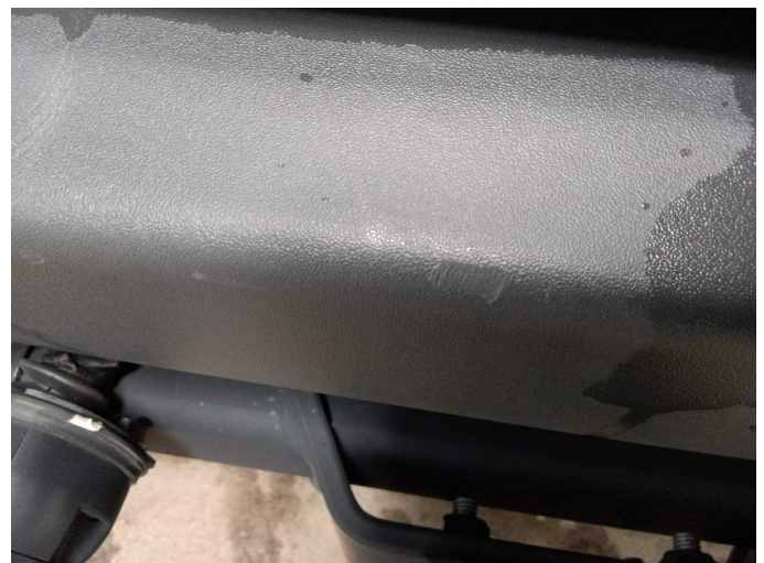
Damage 3: Rear bumper: Rear bumper - Scratched - Replace
