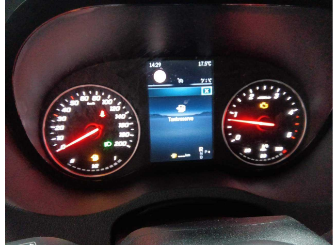
Damage 2: Instrument panel: Indicator light (Motorkontrolleuchte) - on - Perform diagnosis
