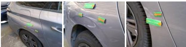
Outer sill R, Dent(s), Replace and paint
