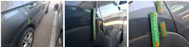
Door RR, Dent(s), Repair and paint (complete)
