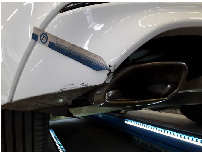
Damage 3: Rear bumper: Rear bumper - Scratched - Paint
