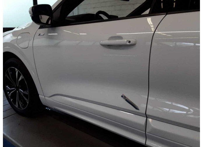
Damage 2: Door - front left side: Door - Scratch(es) - Smart repair
