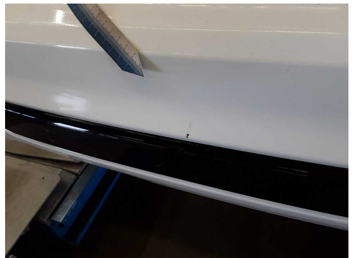
Damage 3: Rear bumper: Rear bumper - Scratched - Paint
