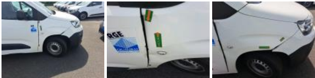
Wing FR, Dent(s) and scratch(es), Replace and paint
