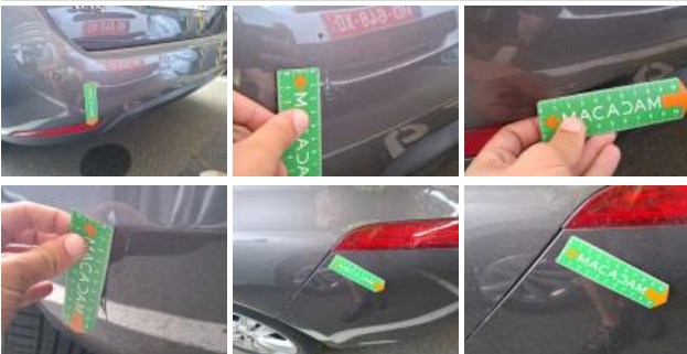
Bumper R, Scratch(es), Repair and paint (complete)
