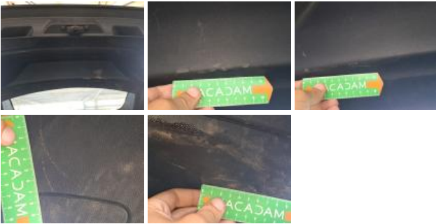
Boot carpet, Deformed / Strained, Replace
