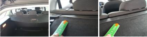
Boot lid covering R, Scratch(es), Replace
