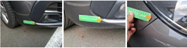
Bumper F, Scratch(es), Repair and paint (complete)
