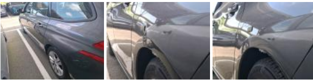
Bumper F, Scratch(es), Repair and paint (complete)
