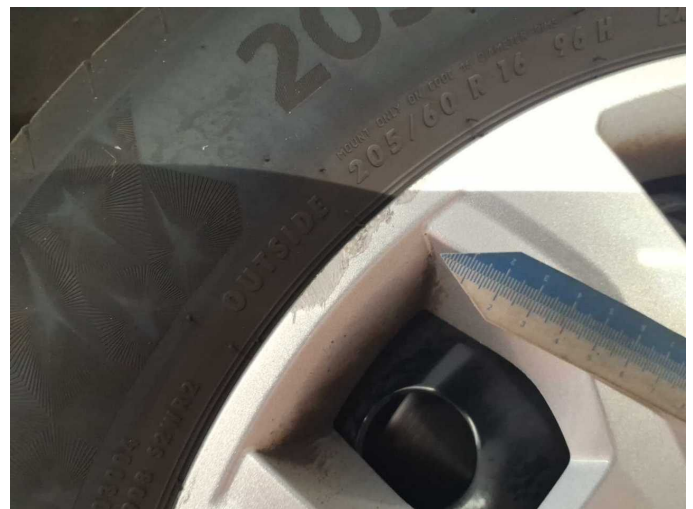
Damage 1: Wheel / tyres: Wheel cover - front right side - Scratched - Loss in value
