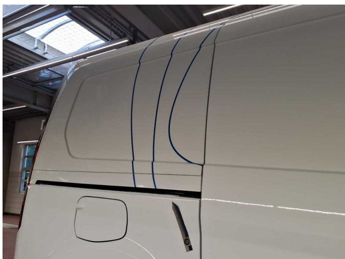
Damage 6: Body: Body - Glued / labelled - De-glue / neutralise
