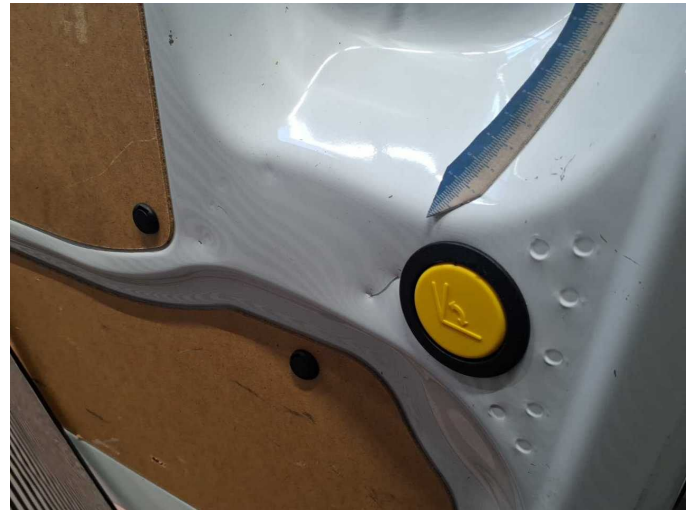
Damage 10: Boot lid / rear door: Rear door - left side - Dent / paintcoat damage - Repair and paint
