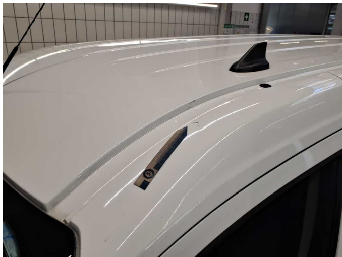
Damage 12: Roof: Roof - Scratch(es) - Paint
