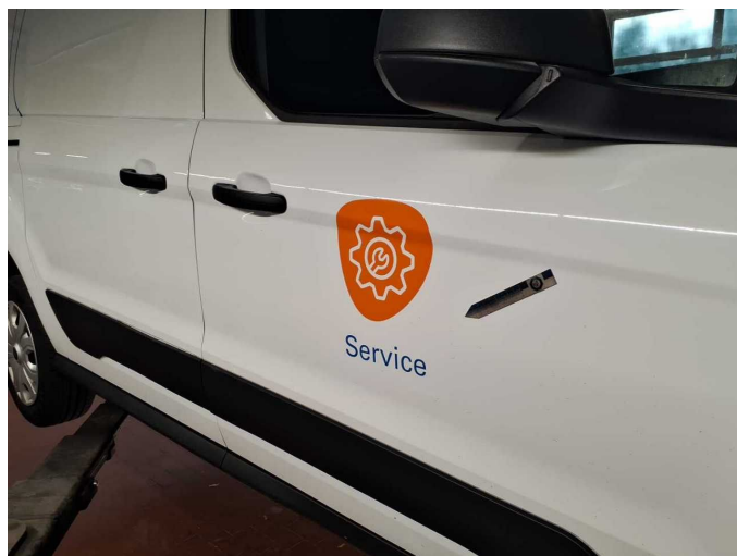
Damage 6: Body: Body - Glued / labelled - De-glue / neutralise
