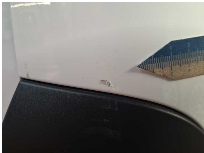
Damage 5: Rear bumper: Bumper - rear right side - Scratch(es) - Smart repair
