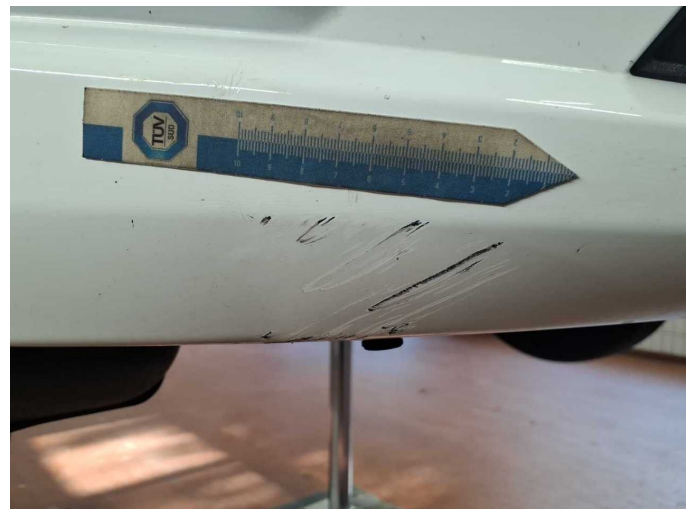
Damage 9: Front bumper: Front bumper - Scratched - Paint
