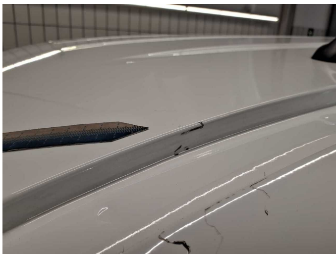
Damage 12: Roof: Roof - Scratch(es) - Paint
