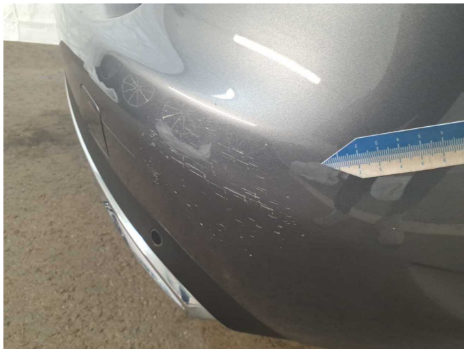
Damage 7: Rear bumper: Rear bumper - Scratched - Paint
