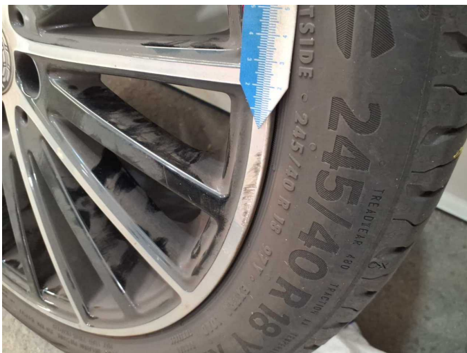
Damage 5: 2nd wheel set: 1 alloy rim (Felge 2. Achse) - Scratch(es) - Loss in value
