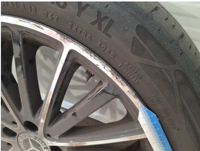
Damage 4: 2nd wheel set: 1 alloy rim (Felge 1. Achse) - Scratch(es) - Loss in value
