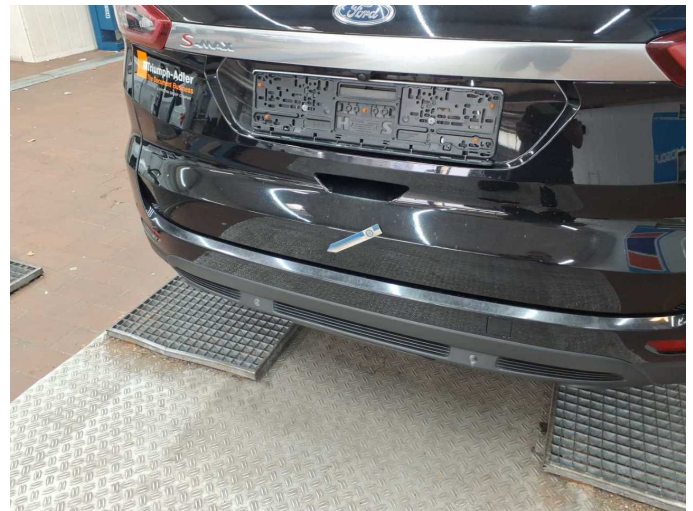
Damage 4: Boot lid / rear door: Boot lid - dent(s) - Loss in value
