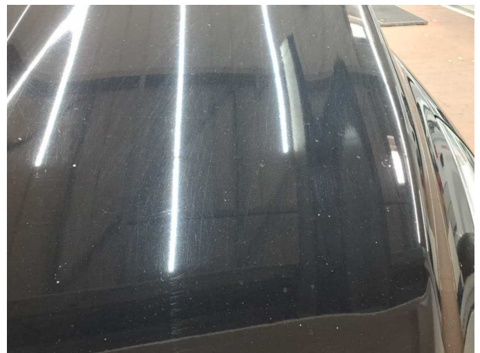
Damage 8: Bonnet: Bonnet - Stone chips - Paint
