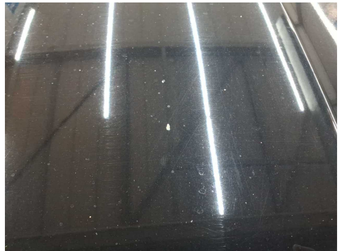
Damage 8: Bonnet: Bonnet - Stone chips - Paint
