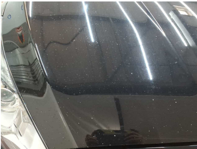
Damage 8: Bonnet: Bonnet - Stone chips - Paint
