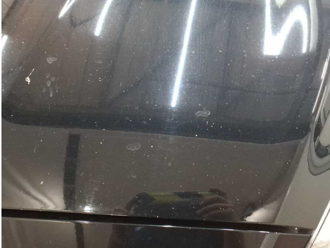
Damage 8: Bonnet: Bonnet - Stone chips - Paint
