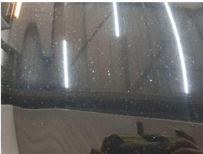
Damage 8: Bonnet: Bonnet - Stone chips - Paint
