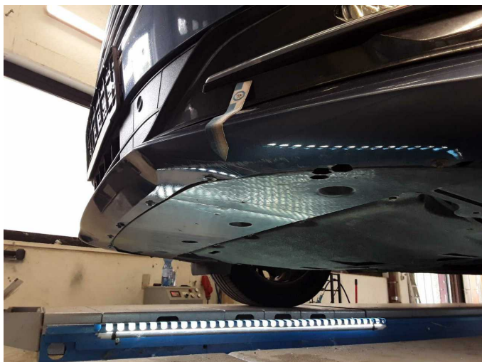
Damage 9: Front bumper: Spoiler - Scratched - Paint
