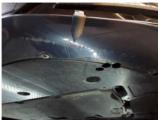
Damage 9: Front bumper: Spoiler - Scratched - Paint
