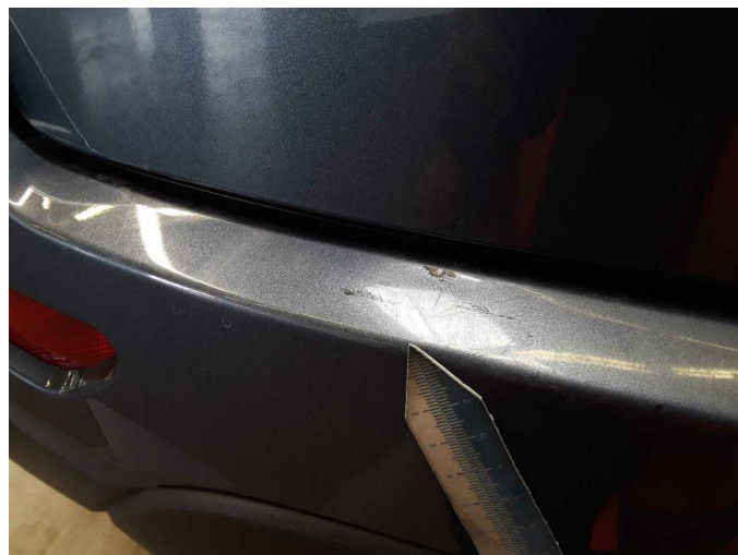
Damage 12: Rear bumper: Rear bumper - Scratch(es) - Paint
