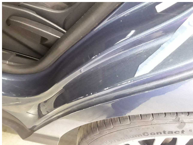
Damage 10: Side panel - rear left side: Elbow - Scratch(es) - Paint
