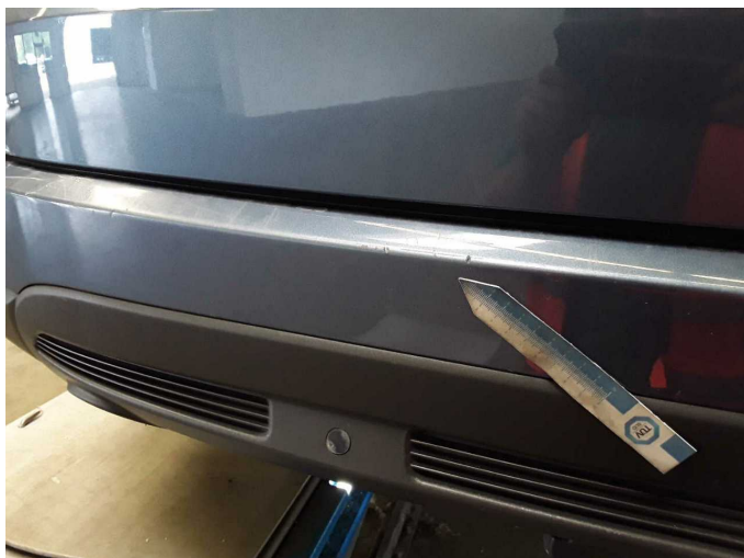
Damage 12: Rear bumper: Rear bumper - Scratch(es) - Paint
