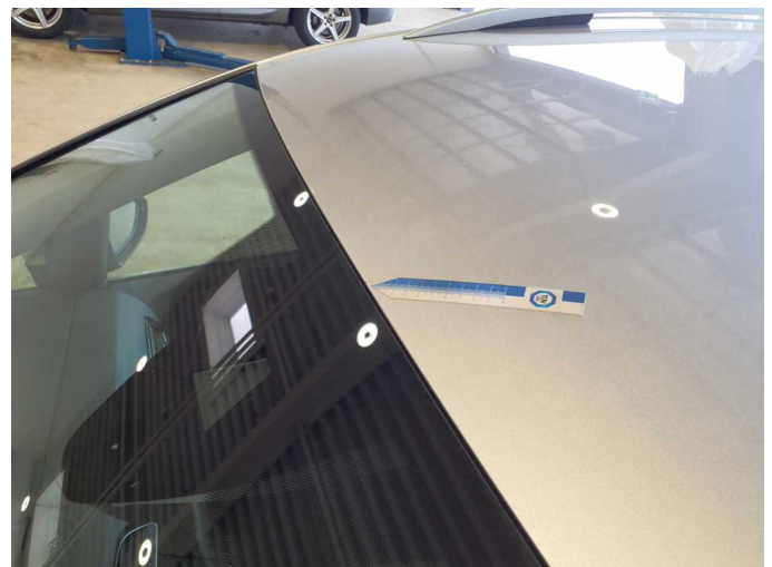
Damage 5: Roof: Roof - Corrosion - Repair and paint
