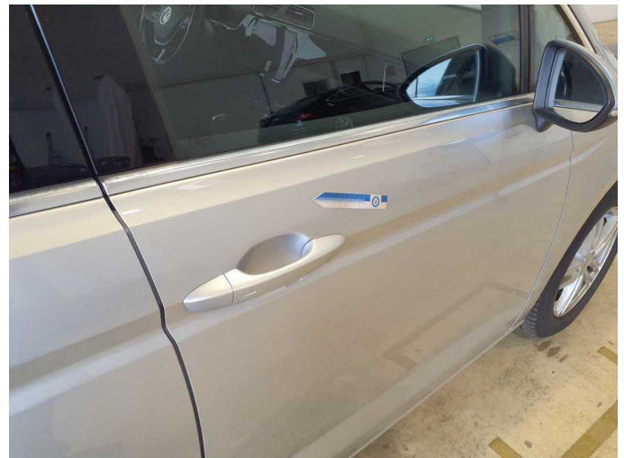
Damage 4: Door - front right side: Door - dent(s) - Repair and paint
