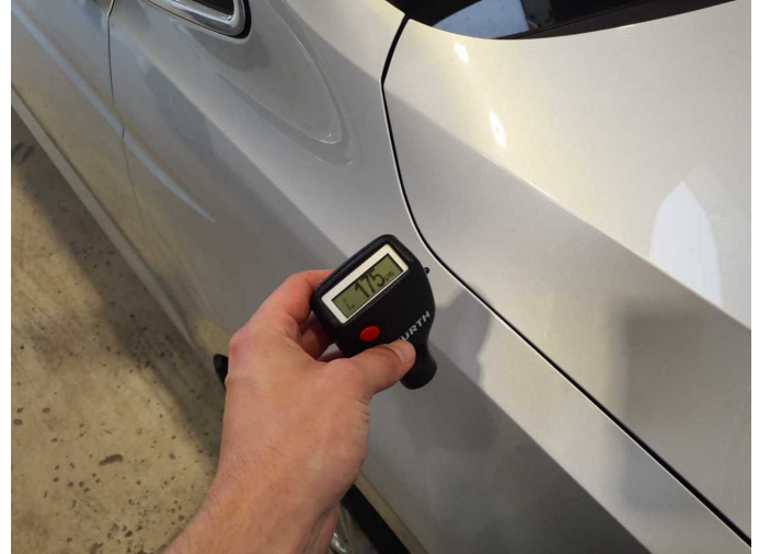
Repainting 1: Mudguard - right side, Door - rear right side, Door - front right side
