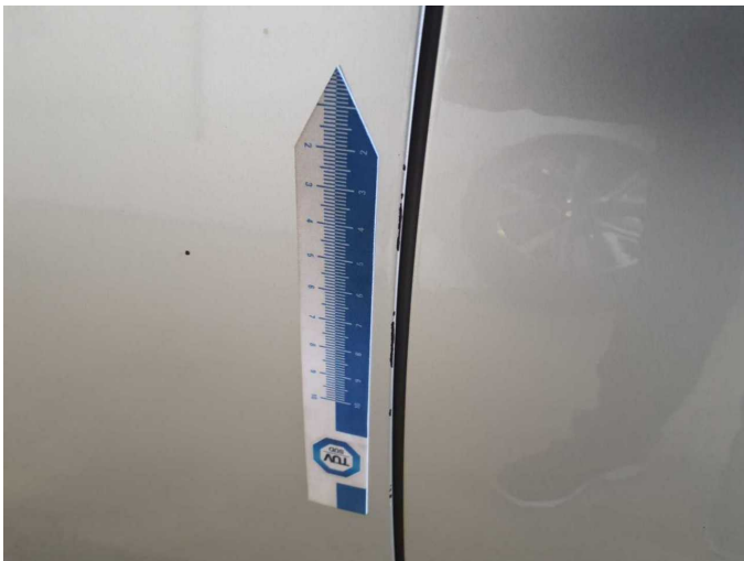
Damage 1: Door - front left side: Door edge - Scratched - Smart repair
