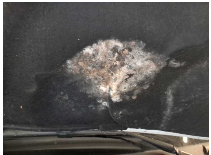
Damage 2: Bonnet: Insulation lining - Soiled - Replace
