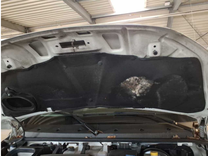
Damage 2: Bonnet: Insulation lining - Soiled - Replace
