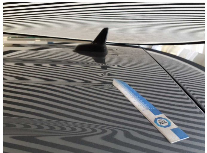
Damage 3: Roof: Roof - dent(s) - Smooth repair work
