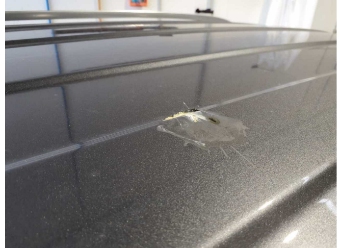
Damage 2: Roof: Roof - Paint defect - Conditioning
