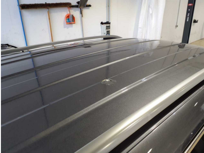
Damage 2: Roof: Roof - Paint defect - Conditioning
