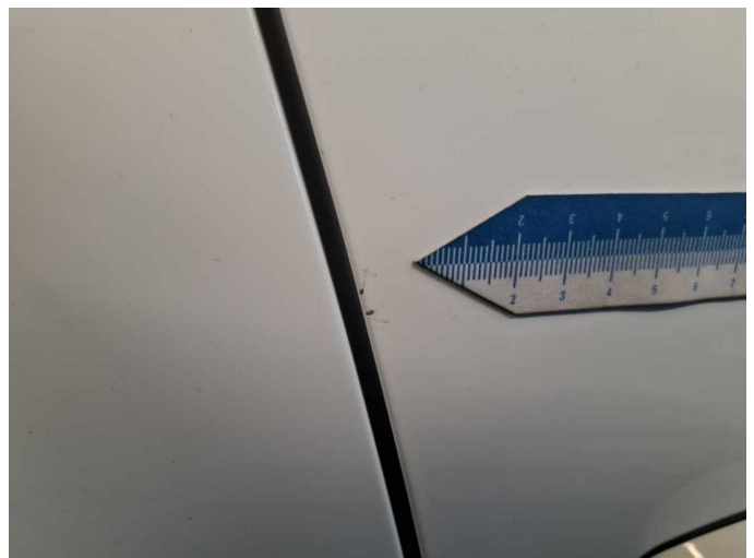
Damage 2: Door - front right side: Door edge - Scratched - Smart repair
