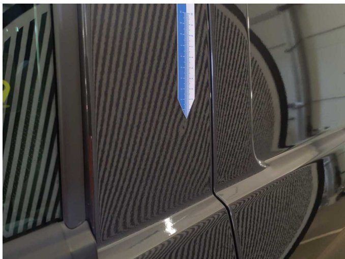
Wear and tear 2: Door - front left side: Door - dent(s) - No deduction
