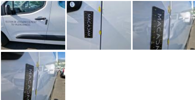
Side panel L, Dent(s), Repair and paint (complete)
