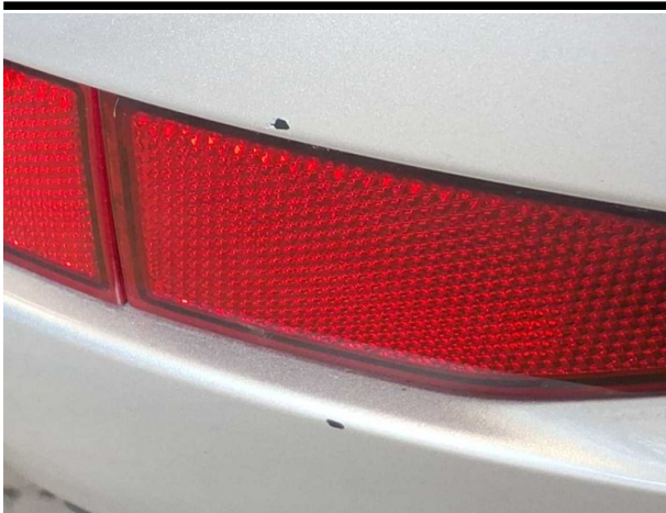
Damage #2: Rear bumper: Rear bumper - Scratch(es) - Repair and paint
