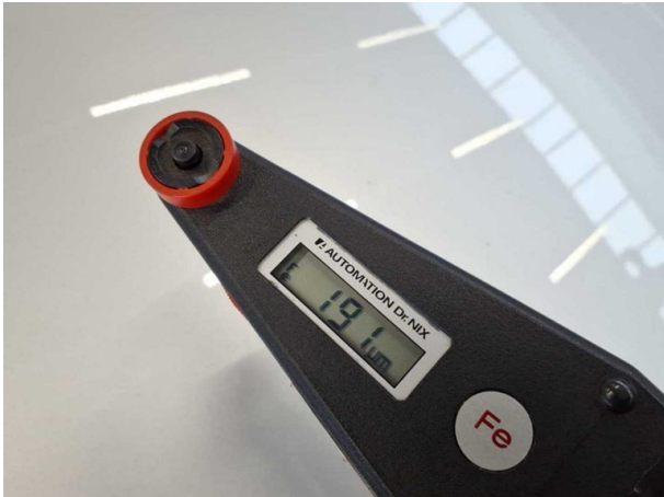
Repainting 1: Mudguard - left side, Door - front left side, Door - front right side
