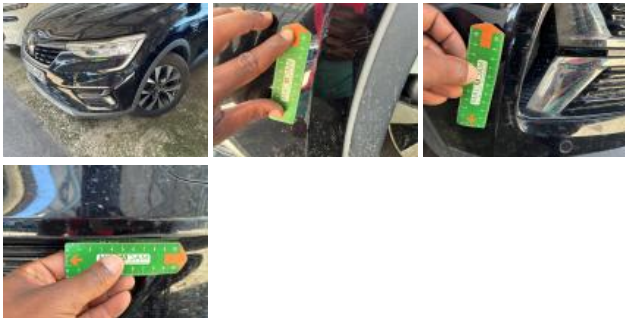
Bumper moulding F, Scratch(es), Replace
