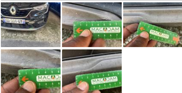
Bumper grille, Broken, Replace
