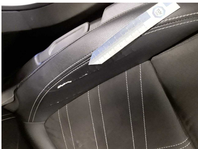
Damage 3: Seat - front: Seat cover - left side - Damaged - Smart repair
