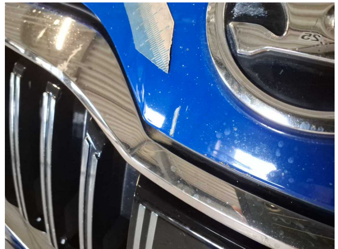
Damage 6: Bonnet: Bonnet - Dent / paintcoat damage - Paint
