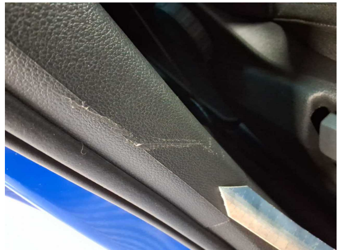
Damage 2: Trim / covers: B-pillar - trim - interior, right side - Scratched - Replace
