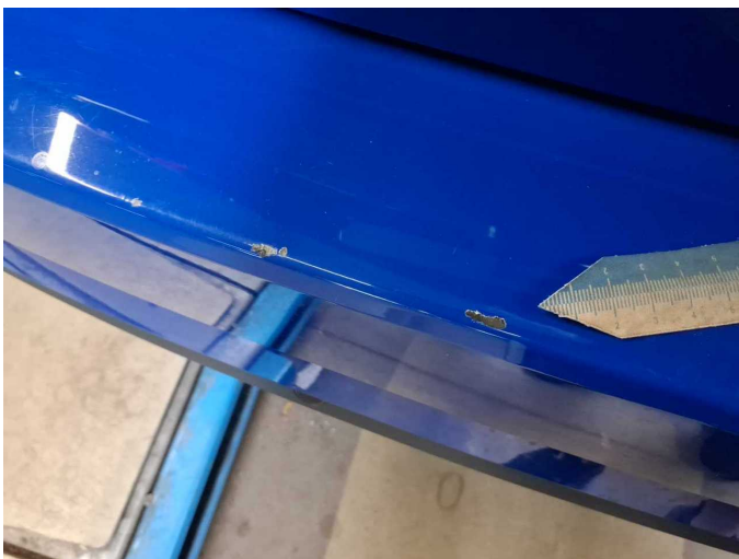
Damage 4: Rear bumper: Rear bumper - Scratched - Paint
