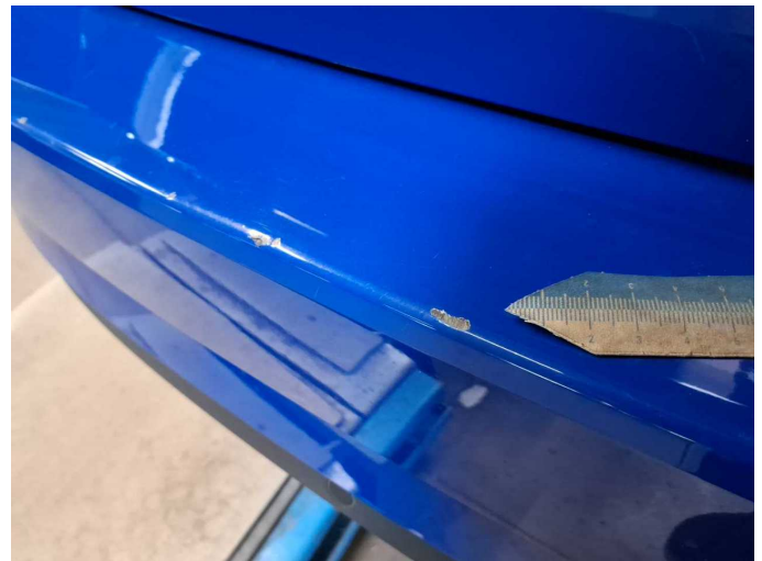
Damage 4: Rear bumper: Rear bumper - Scratched - Paint
