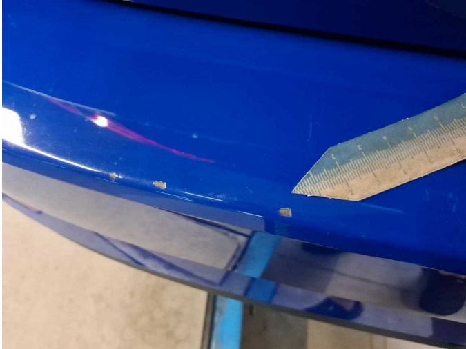
Damage 4: Rear bumper: Rear bumper - Scratched - Paint
