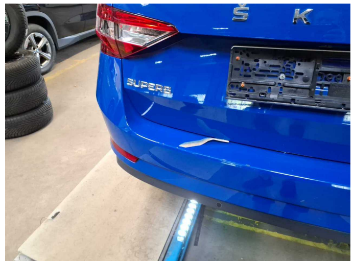
Damage 4: Rear bumper: Rear bumper - Scratched - Paint
