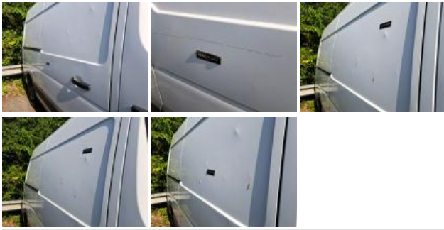
Central pillar R, Dent(s), Repair and paint (complete)
