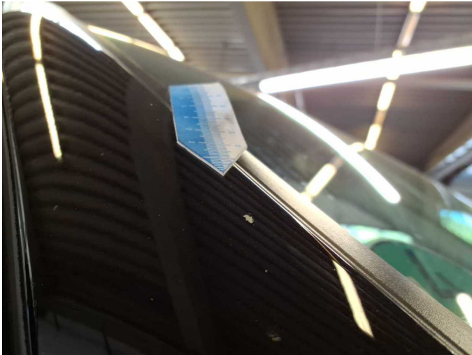
Wear and tear 4: Roof: Roof rail - right side - Stone chips - Smart repair
