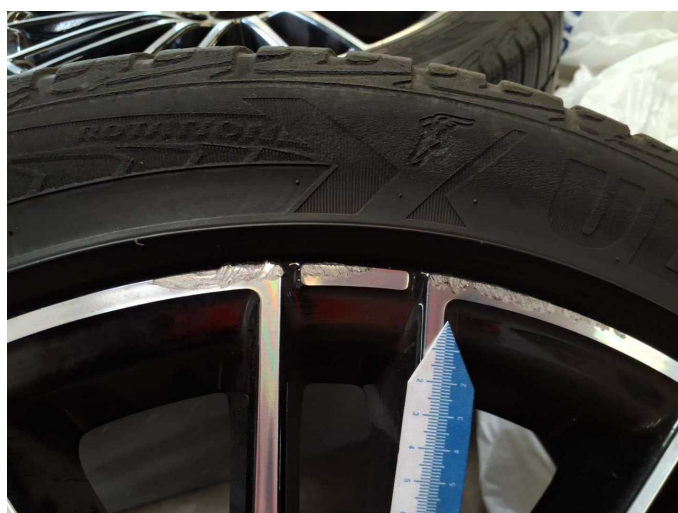
Damage 16: 2nd wheel set: 1 alloy rim - Scratched - Replace
