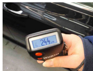
Paint thickness Door FR
