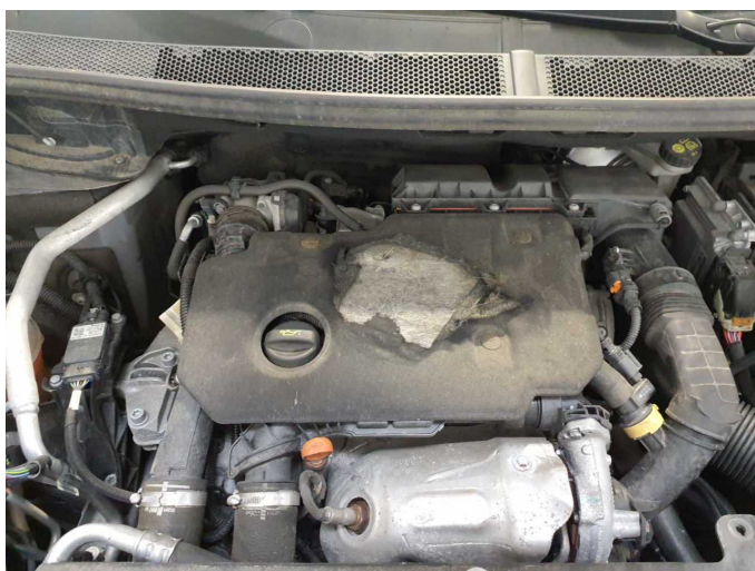
Damage 14: Engine: Engine cover - Damage caused by marten / rodent - Replace
