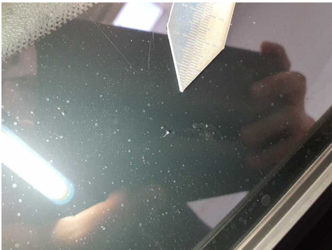
Damage 18: Vehicle glazing: Windscreen (Randbereich) - Stone chips - Replace
