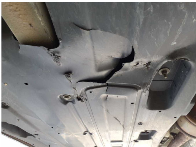
Damage 15: Body: Underbody panelling - Broken / torn - Replace
