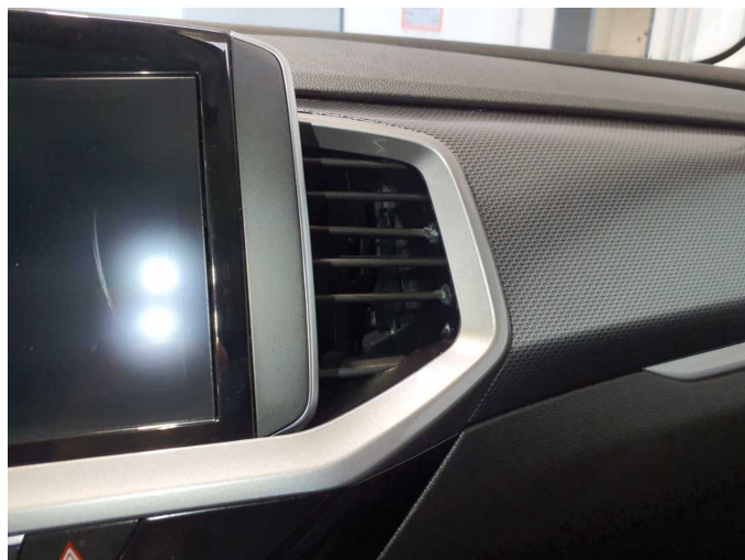
Damage 12: Instrument panel: Air nozzle - centre - Broken / torn - Replace
