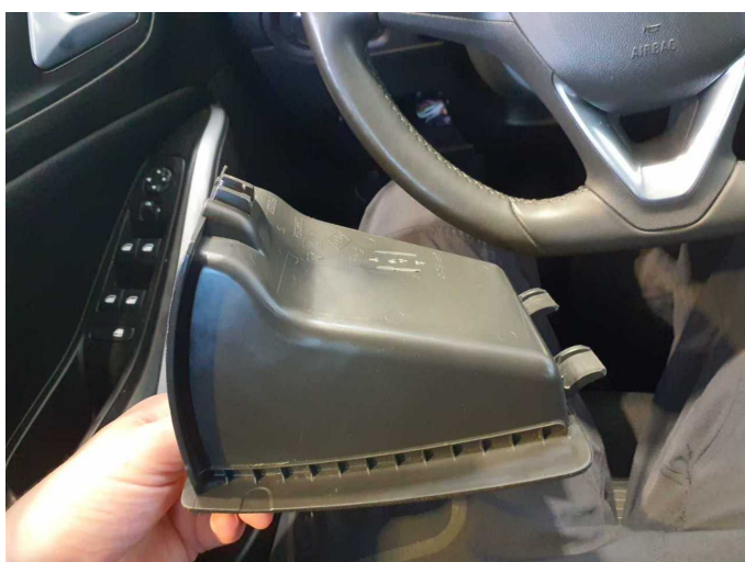
Damage 10: Trim / covers: Trim / covers (Ablagefach) - Broken / torn - Replace
