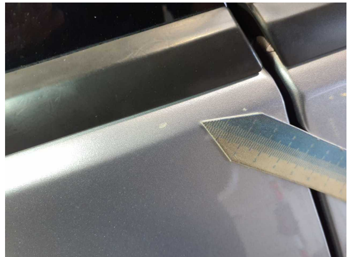
Wear and tear 2: Door - rear left side: Door - Stone chips - No deduction
