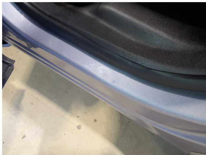
Damage 3: Side panel - rear left side: Sill - dent(s) - Smooth repair work
