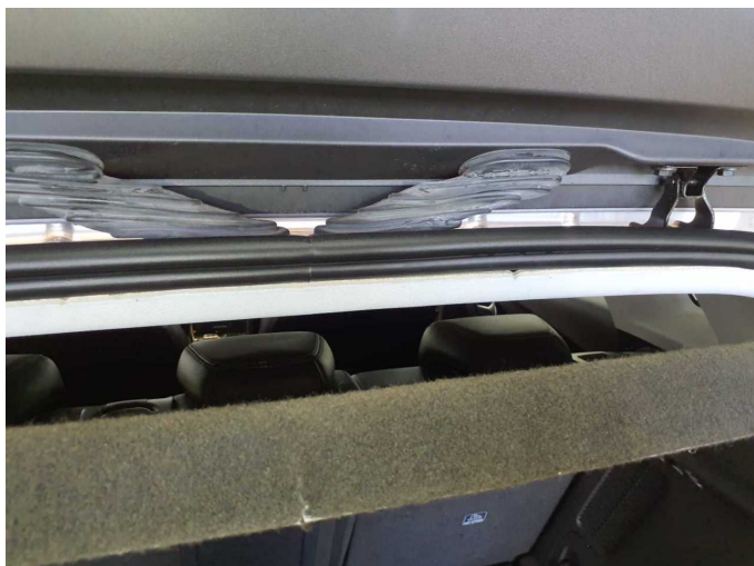
Damage 6: Trim / covers: Roof lining - Loose - Repair
