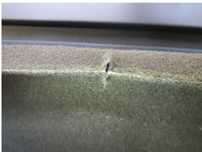
Damage 16: Interior: Boot cover / roller cover - Broken / torn - Replace
