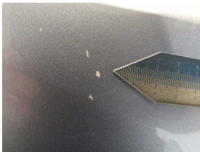
Damage 17: Bonnet: Bonnet - Corrosion - Paint
