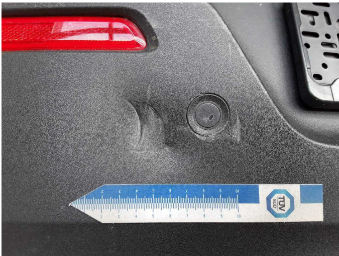
Damage 5: Rear bumper: Spoiler - Deformed - Replace
