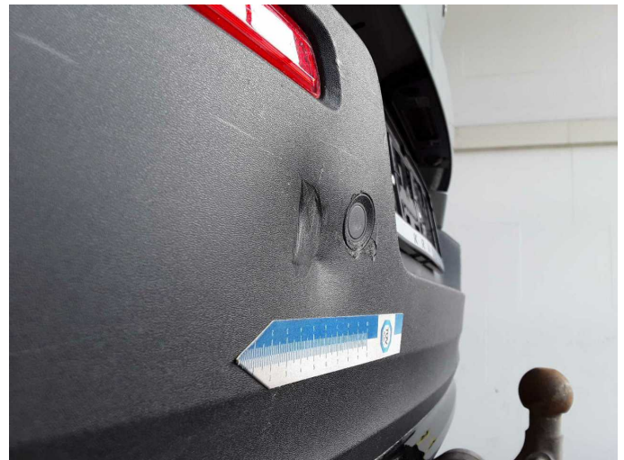
Damage 5: Rear bumper: Spoiler - Deformed - Replace
