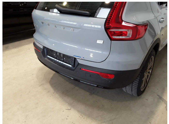
Damage 4: Rear bumper: Bumper - rear right side - Scratch(es) - Smart repair
