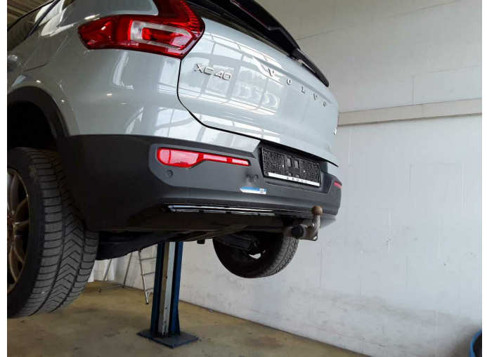
Damage 5: Rear bumper: Spoiler - Deformed - Replace
