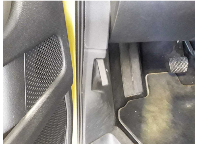
Damage 1: Bonnet: Handle - engine hood release cable - Differs from the original configuration - Perform diagnosis
