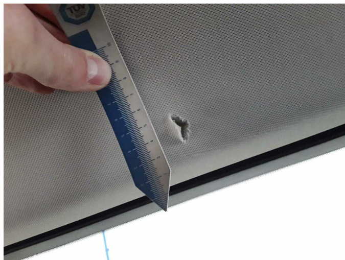
Damage 4: Trim / covers: Roof lining - Broken / torn - Replace
