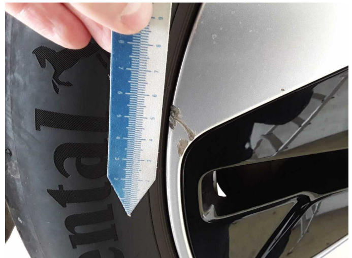
Damage 2: Wheel / tyres: Alloy rim - front right side - Scratch(es) - Loss in value
