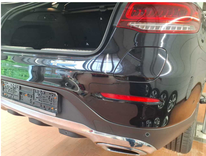
Damage 8: Rear bumper: Rear bumper - Scratched - Paint
