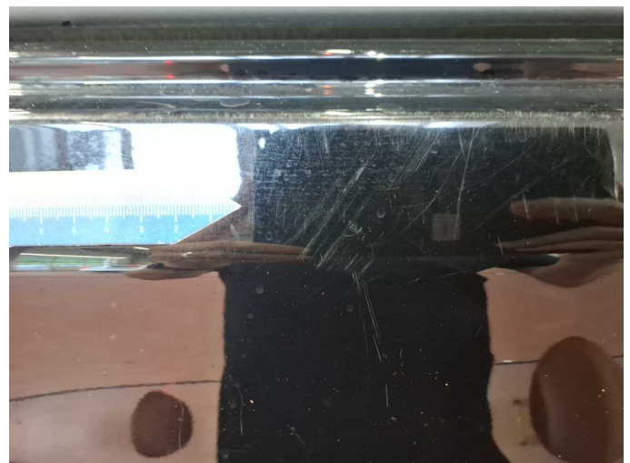
Damage 8: Rear bumper: Rear bumper - Scratched - Paint
