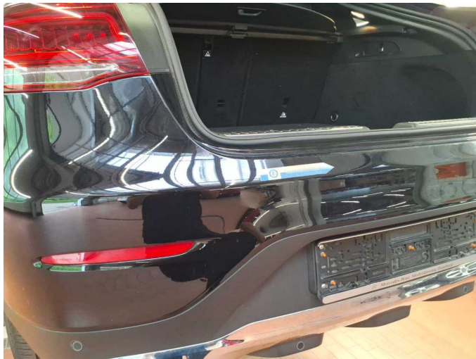
Damage 8: Rear bumper: Rear bumper - Scratched - Paint
