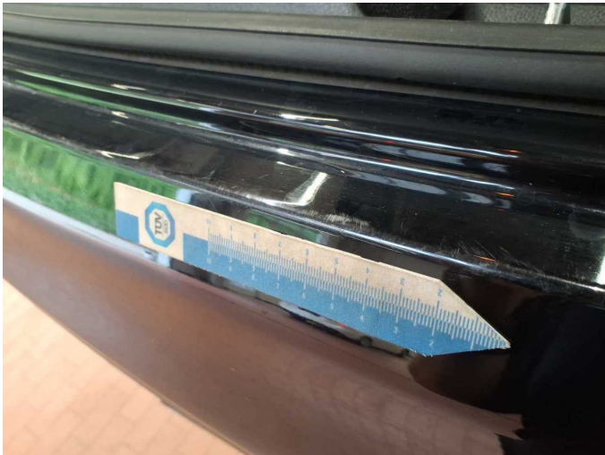
Damage 8: Rear bumper: Rear bumper - Scratched - Paint
