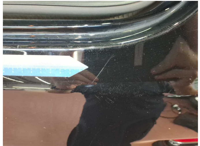
Damage 8: Rear bumper: Rear bumper - Scratched - Paint
