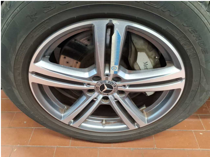
Damage 4: Wheel / tyres: Alloy rim - front left side - Corrosion - Replace
