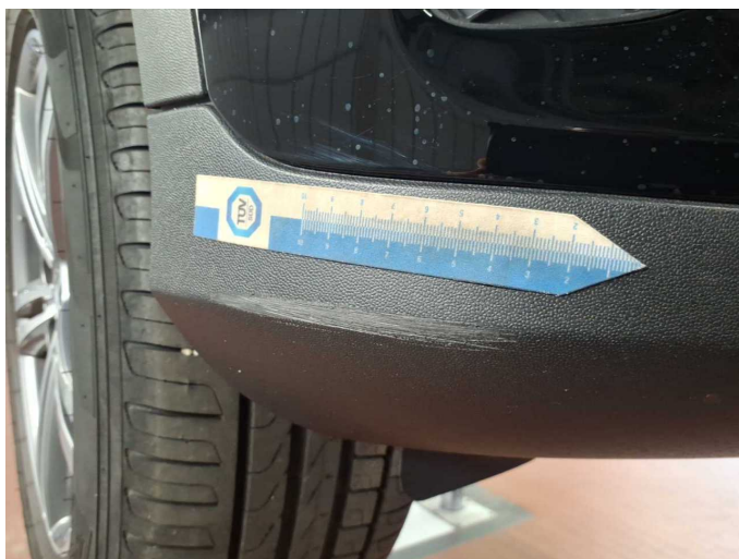
Damage 1: Front bumper: Spoiler - Scratch(es) - Loss in value
