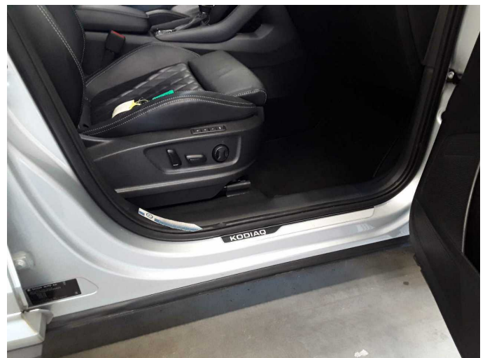
Damage 3: Door - front right side: Door seal - Damaged - Replace
