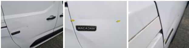
Side wall RR, Dent(s), Acceptable
