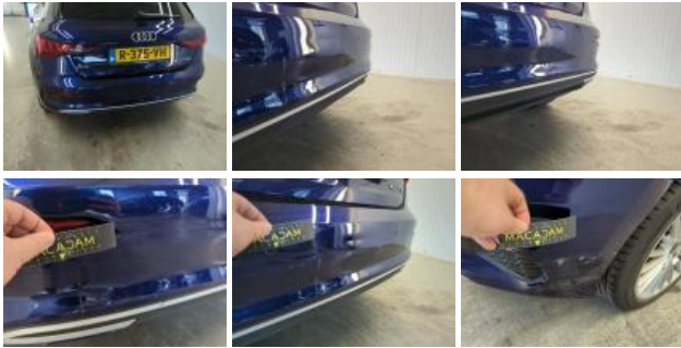
Bumper moulding RR, Broken, Replace
