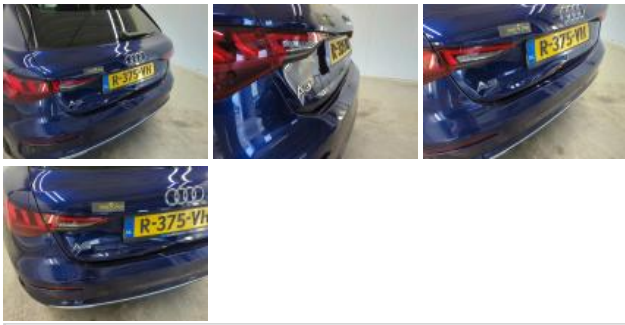
Rear light L tailgate, Broken, Replace
