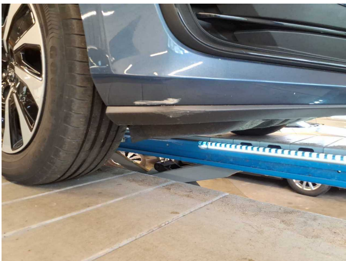
Damage 3: Front bumper: Spoiler (rechts) - Scratched - Replace
