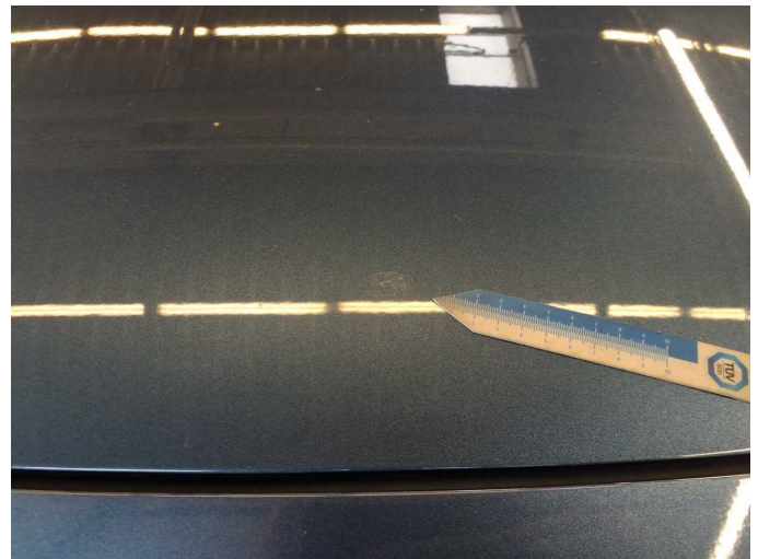
Damage 5: Bonnet: Bonnet (Harzflecken) - Paint defect - Paint
