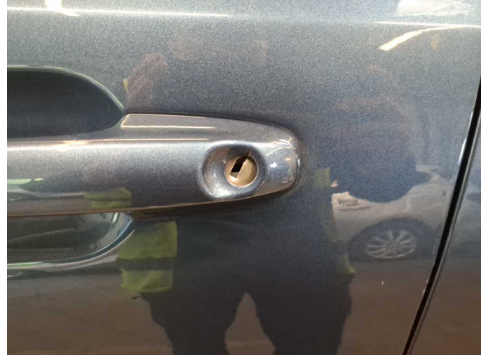
Damage 4: Door - front left side: Lock / Locking mechanism - Damaged - Replace
