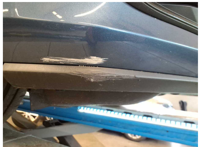
Damage 3: Front bumper: Spoiler (rechts) - Scratched - Replace
