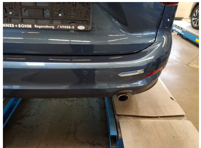
Damage 6: Rear bumper: Rear bumper (inkl. Abdeckung) - Scratched - Repair and paint
