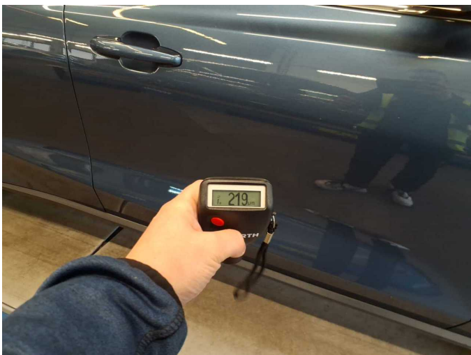
Repainting 1: Door - front right side
